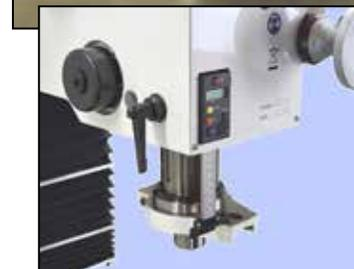
Figure 2 **DRO, depth stop & quill locking lever**
