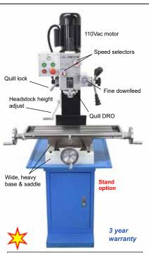
Single speed ac motor with 6 speed gearbox. Great value for a machine of this weight (200 lbs heavier than the PM-25MV-BD).
