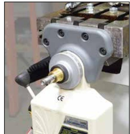
**Figure 6 Dial & knurled collar installed**
