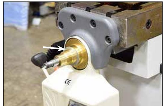
**Figure 5 Bevel gear installed**
