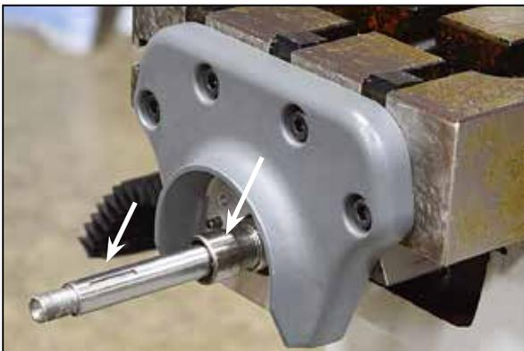
**Figure 3 Support casting installed**
