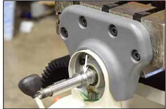
**Figure 4 Feed motor installed**
