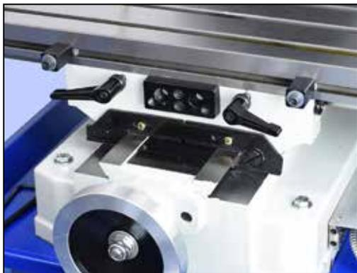
**Figure 8 Install the limit switch backing plate**
