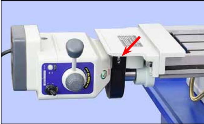
**Figure 7 Install the power feed unit**
