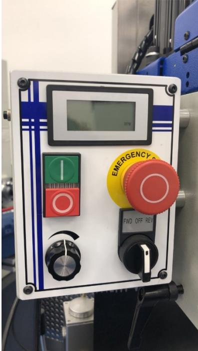
Step 5: Press the Green Power Button, the display and the programmer should light up as shown below.
