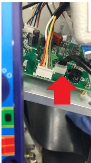
Step 4: Make sure the FWD/REV switch is in the OFF position, and the E Stop is out
